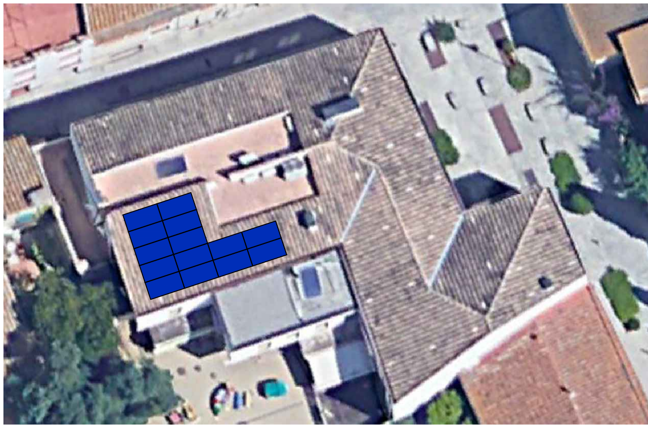
CAN ROSTOLL: 6.300 Wp
