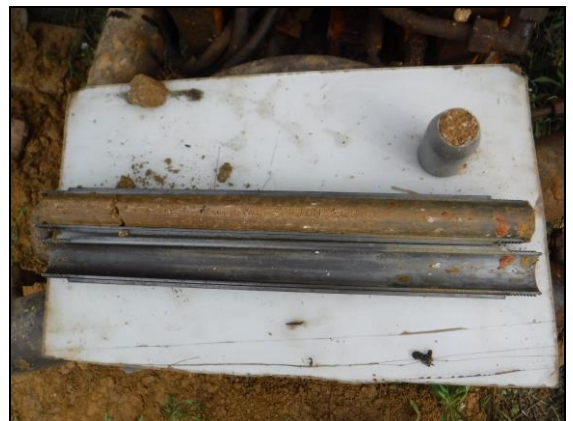
Foto 4: Sondeig S-1, SPT a 8,0 metres.
