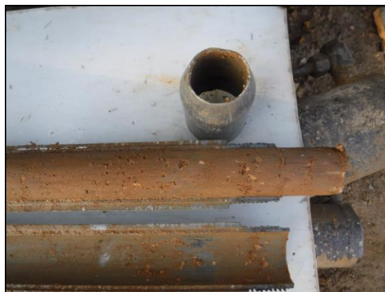
Foto 44: Sondeig S-13, SPT a 5,0 metres.
