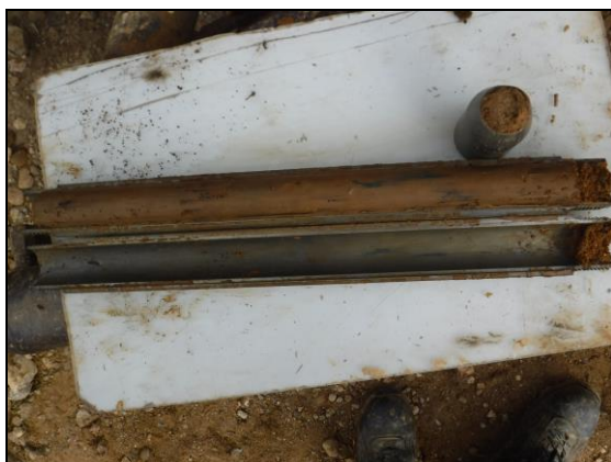
Foto 51: Sondeig S-15, SPT a 1,0 metre.
