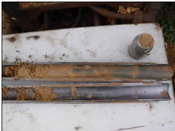
Foto 7: Sondeig S-2, SPT a 7,0 metres.
